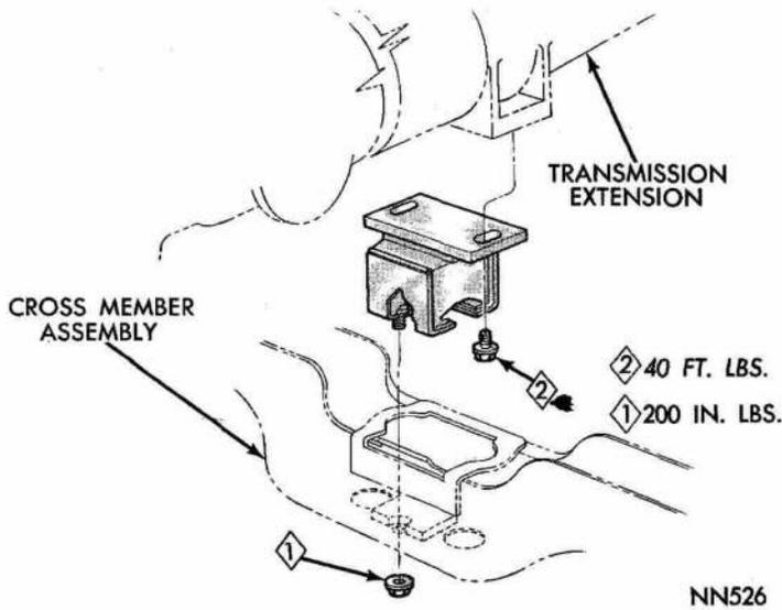
**Fig. 4—Engine Rear Support (115.5" and 116.5" Wheelbase with 4-Speed Transmission)**
